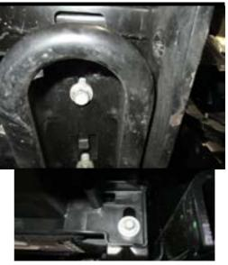
We recommend that the 15mm head tie down/recovery loop bolts have loctite 243b thread lock added to them on assembly, this is not included with the product.
